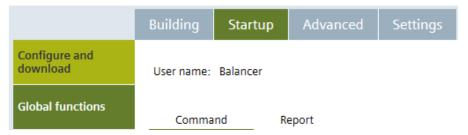
**4.2** Select **Air Balancer Commanding List** from the Command list dropdown and tick the checkboxes next to parameters to be previewed and eventually commanded.
