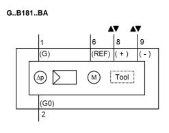
Tool = Configuration and maintenance interface (7-pin)
