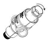
Loosen the differential pressure regulator until the marking on the regulator is aligned against the flow direction
