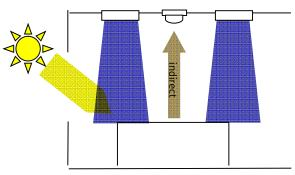
For indirect brightness measuring a maximal distance of 2.8 m is recommended. In case of larger distances the measuring can be realized via a reference area with 2.8 m distance.
