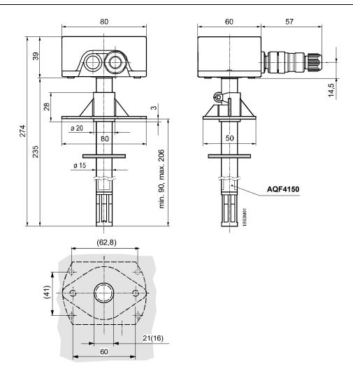
Drilling template with (without) mounting flange
