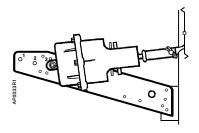
Figure 6. Frame Mounting, Normally Closed Damper.
