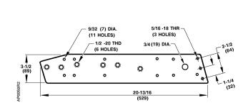
Figure 11. Actuator Mounting Plate 331-623. Dimensions in Inches (Millimeters).
