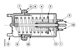
Figure 1. Standard Actuator.
