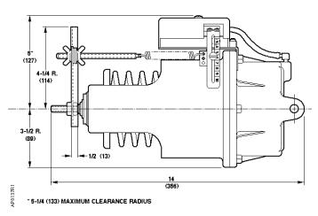
Figure 12. No. 6 Actuator with the RL 147 Positioning Relay Mounting. Dimensions in Inches (Millimeters).
