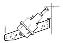
Figure 5. Frame Mounting, Normally Open Damper.
