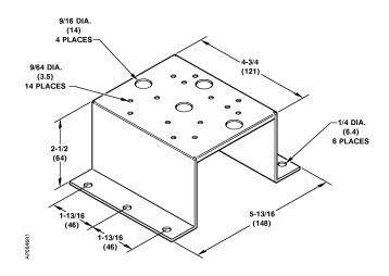
Figure 10. Offset Mounting Bracket 333-176. Dimensions in Inches (Millimeters).
