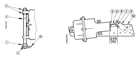
Figure 2. Extended Shaft/Frame Mounting Actuator Assembly.
