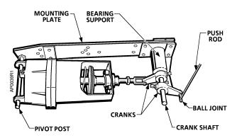
Figure 3. Remote Mounting Kit 331-618 with 331-2856 Actuator Mounted.
