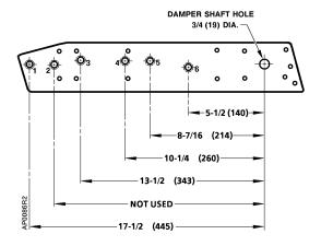
Figure 7. Actuator Mounting Plate 331-623
