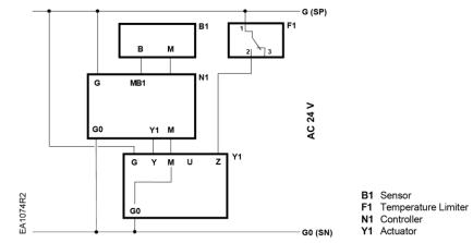
Figure 14. Connecting Terminals.
