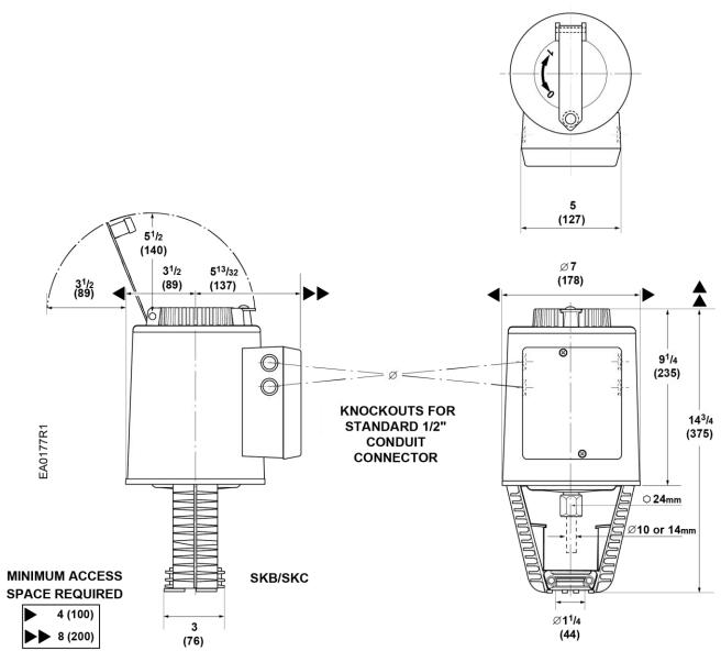
Figure 18. Dimensions of SKB/C in Inches (Millimeters).
