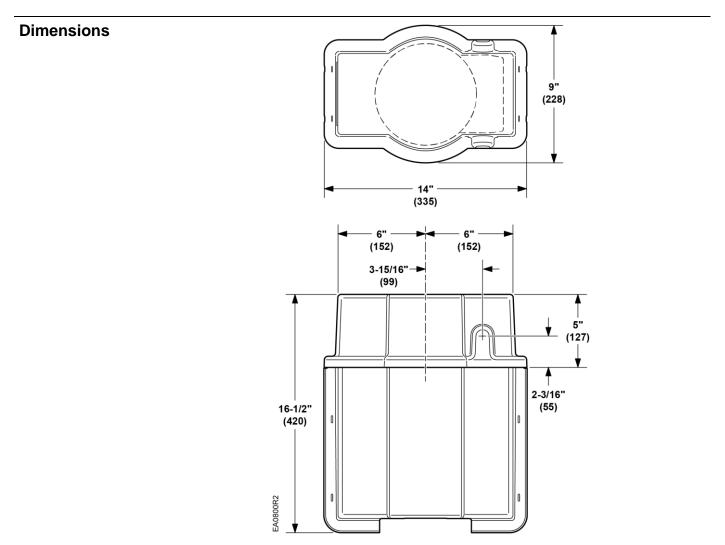
Figure 17. Dimensions of the 599-10065 Weather Shield in Inches (Millimeters).
