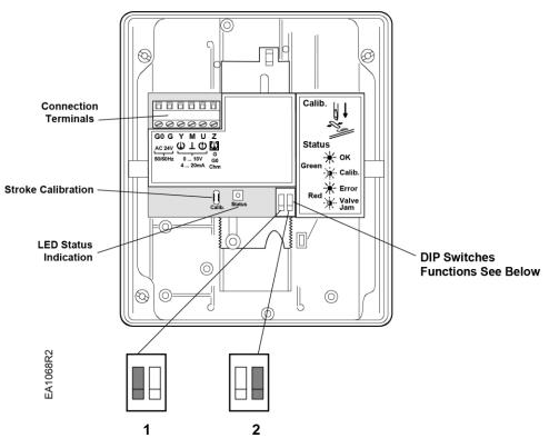
Figure 10. DIP Switches.
