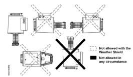
Figure 7. Acceptable Mounting Positions.
