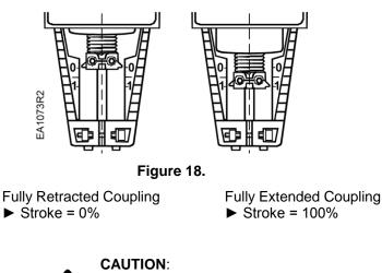
The manual adjuster must be rotated counterclockwise to the end stop until the red indicator marked MAN is no longer visible.
