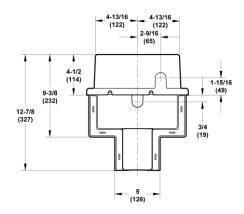
Figure 24. Dimensions of 599-10071 SKD Weather Shield in Inches (Millimeters).
