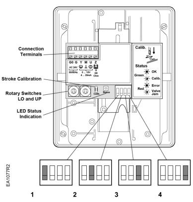
Figure 13. DIP Switches.
