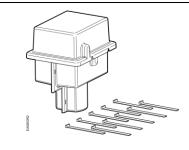
**599-10071** The SKD actuator is UL listed to meet NEMA TYPE 3R requirements (a degree of protection against rain, sleet, and damage from external ice formation) when installed with this weather shield and outdoor-rated conduit fittings in the vertical position. See *Service Kits* for replacement ultraviolet resistant cable ties.
