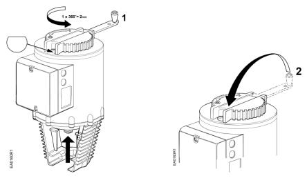
Figure 17. SKB/C Automatic Operation.
