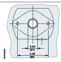
Figure 10. Drilling Pattern.
