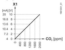
Figure 1. CO<sub>2</sub> Signal Output (X1).
