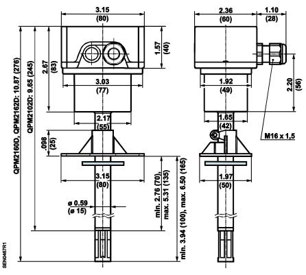
Figure 9. QPM Series Duct Air Quality Sensors with Display.
