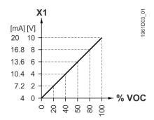
Figure 2. VOC Signal Output (X2).
