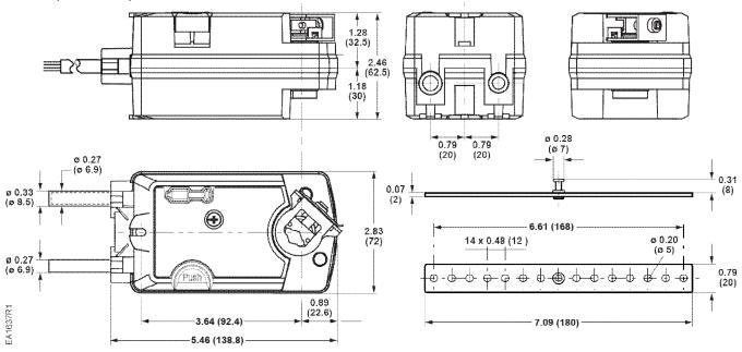
Figure 9. GSD Series Damper Actuator.
