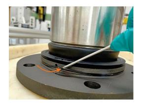
3 Check choke plug is in position. Lubricate O-ring with supplied grease. Put on new O-ring into the O-ring groove of the flange plate. See notes 1-3 below for more details.
