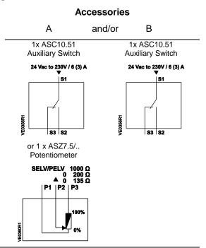
The diagram shows all possible connections. The application determines which connections are used.
