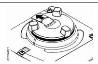
When the black slide switch is pushed out, the manual adjuster remains engaged.
