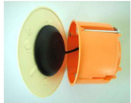
Mounting patch antenna
