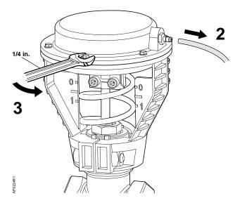
Figure 2. Remove and Cap the Air Line. Remove the Actuator Upper Housing.
