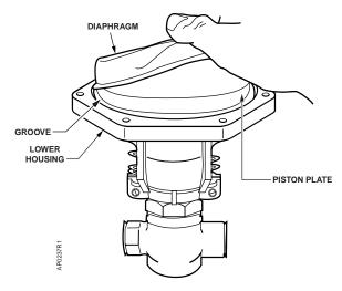
Figure 6. Replacing the Diaphragm on a Powertop Actuator.
