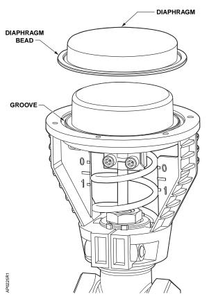
Figure 3. Remove and Replace the Diaphragm.
