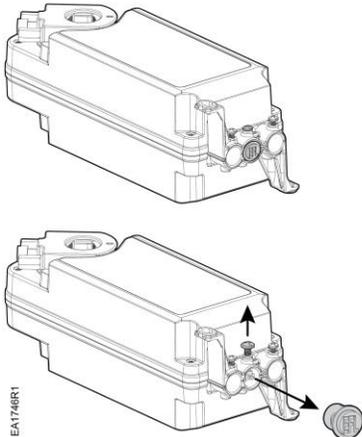
**Figure 8. Removing the EFL.**
