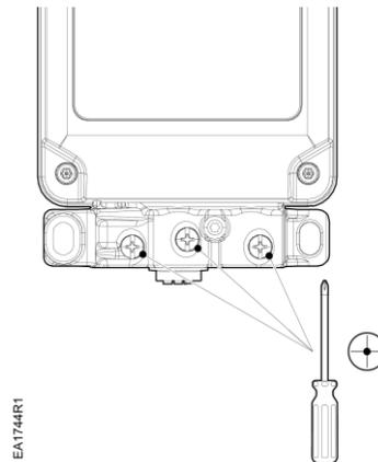
**Figure 7. Tighten Conduit Screws (No. 2 Phillips Screwdriver).**
