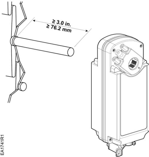
**Figure 3. Shaft Length and Proper Shaft Adapter Location.**
